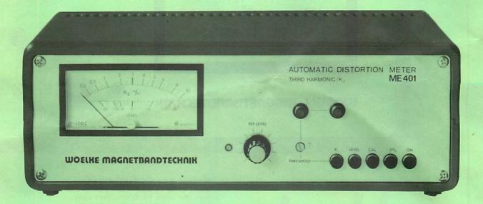
The ME 401: a completely new automatic, direct reading, third harmonic distortion analyzer for alignment of studio tape recorders as well as consumer cassette decks. The ME 401 is a development resulting from experiences gained in manufacturing test equipment for quality control, repair and service labs. It is another in the well known ME series of test equipment made by the Woelke organization.
