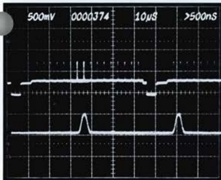
Fig. 3: Digital Delay Analog-Delay operation. The 7D11 triggers Time Base A at the beginning of the 374th line (upper trace). The 7th and 8th vertical bars are intensified by Time Base B set by the 7B71 delay time multiplier. The lower trace shows video information on the B delayed sweep.
