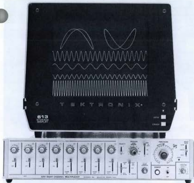
The 4701 Eight-Channel Multiplexer and the 613 Storage Display comprise a system capable of portraying eight different signal sources.
