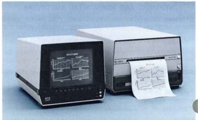
The 613 Storage Display is fully compatible with the 4610 Hard Copy Unit.
