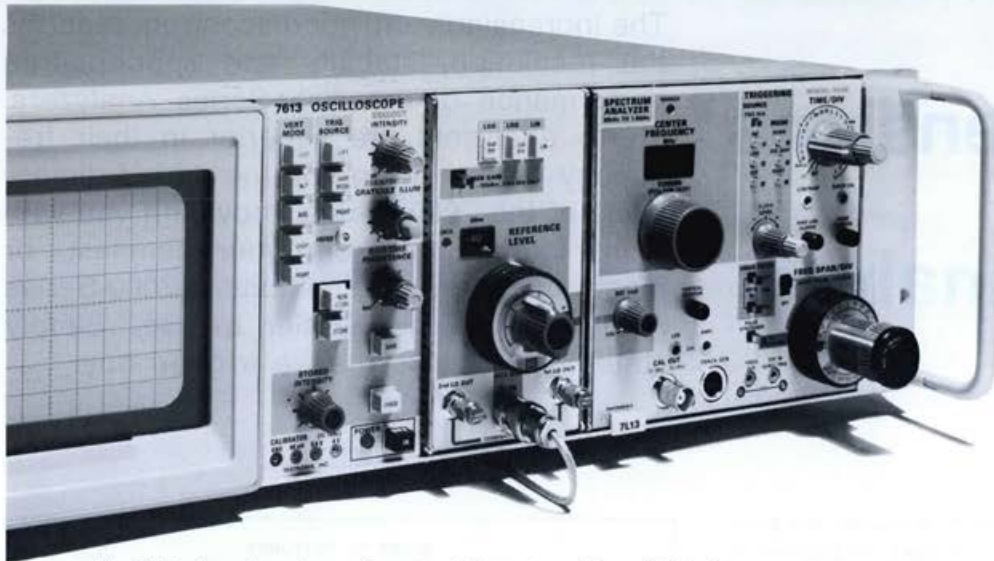
The 7L13, shown here in a rackmount mainframe, is a "three-wide" unit.
