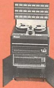
DC servo capstan with external control capability • Selectable 7-1/2, 15, 30 ips speeds • 5 to 45 ips variable speeds • Complete mode-to-mode logic • 50-60 Hz, 110V or 220V input overseas application • Power failsafe • Edit capability • Remote transport control • Selectable wind mode tensions.
