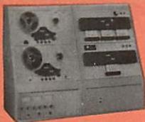
Modular design allows mixing of components for cassette to cassette, reel to cassette, reel to reel or even cassette to reel tape duplication. Two speed hysteresis synchronous motor drive, open reel master 15 and 30 ips, other transports 7-1/2 and 15 ips. Solid state plug-in electronics. Available for various track, channel and power requirements.
