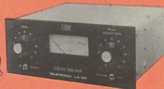
The LA-3A Solid State Leveling Amplifier, maintains characteristics of the T4A electro-optical attenuator. Independent gain reduction control provide for setting of the limiting of compressing action, and the system gain. Adjustable limiting frequency response allows 10 dB increase in gain reduction at 15 kHz compared to frequencies below 1 kHz,
