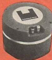
Intended for use where high sound pressure levels must be generated, these compression drivers utilize phenolic impregnated linen diaphragms and edgewound ribbon voice coils to provide maximum power capacity and conversion efficiency. The 2482 is capable of generating extremely high sound pressure levels while maintaining crisp, natural reproduction of speech. Power Cap: 120 watts; Freq. Range: 300-6 kHz; Crossover Freq: 300 Hz.
