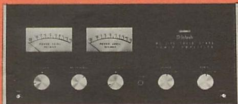
MC 2105 Power Output 105 watts minimum sine wave continuous average power output, per channel, both channels operating into 4 ohms, 8 ohms, or 16 ohms load impedance Output Load Impedance 4 ohms, 8 ohms, or 16 ohms; separate terminals are provided for each output Rated Power Band 20 Hz to 20,000 Hz Total Harmonic Distortion 0.25% maximum harmonic distortion at any power level from 250 milliwatts to 105 watts per channel from 20 Hz to 20,000 Hz, both channels operating.
