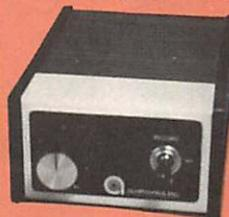
AUDITRONICS Tape to Telephone Record/Play adaptor Model TA-1 is designed to facilitate tape recording from a conventional telephone line. Also, recorded material may be played through the adaptor into the same telephone line. A simple two-wire connection is made between any ordinary telephone and the adaptor. One connection to recorder line-in and a second from recorder line-out, or speaker/headphone output, completes the hookup. (3-1/2 foot cables supplied)
