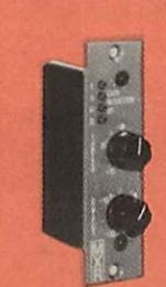
The MXR Mini Limiter is designed as a cost-effective answer to meeting the wide variety of audio limiter applications. Low noise, low distortion and quick response enable it to effectively control signal peaks. Attack time is fast (approx. 1 ms.), and release time is both variable via rear trim pot and dependent upon the amount of gain reduction. Four instantly responsive L.E.D.'s continuously indicate gain reduction.
