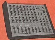
Model ESC-8, the Eight Pack, is a portable eight channel stereo mixing console that features low distortion (less than 0.1%) and low noise (-123 dBm equivalent input noise) as well as balanced low impedance inputs and variable input gain. The ESC-8 has extensive control features including separate monitor mix, pan, high and low equalization, and overload indicators on each channel. It also has a 9 Watt headphone amp, an internal reverb unit, and two accurate peak reading level meters.
