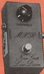
The primary function of the Noise Gate/Line Driver is that of removing unwanted noise from any musical performance by gating off any signal below a variable threshold level. The threshold control allows the musician to adjust the level at which the Noise Gate cuts off, removing unwanted noise between notes, and at the end of performances.
