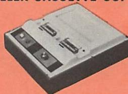
Desk top cassette copier for use by non-technical personnel. Simple two button operation (Rewind & Copy) with track selector for copying track 1 or track 2 or both. Add-on capabilities. Automatically turns on with insertion of original cassette, automatic rewind after copying is completed and automatically shuts off when original cassette is removed. Duplicating speed—30 ips, rewind speed—60 ips. Companion slave available.
