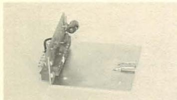
Modification groups mounted on screw holes "A" with wires to terminal side of receptacle. Wires are soldered to appropriate terminals on receptacle.
