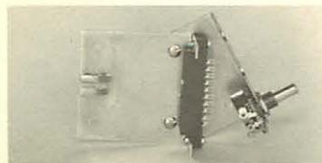
Mounting bracket BKT 4000 is used wherever it is necessary to mount the TRY 4000 on a non-horizontal plane. The TRY 4000 may be mounted in any one of four attitudes, rear down, front down, either side down. In addition, one or two rotary controls may be mounted on BKT 4000 and the assembly may be mounted on the bushing of the controls. The BKT 4000 has an angle cut on one side to permit mounting near the bottom of a sloping panel.
