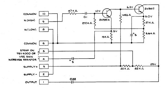
THE AM4300 AMPLIFIER IS PRIMARILY INTENDED FOR USE AS A HIGH-IMPEDANCE MICROPHONE PREAMPLIFIER, but may also be used as a post-mixing amplifier, a post-equalization amplifier, etc. When equipped with Modification Group MG4001, it becomes a phonograph preamplifier with RIAA characteristic.
