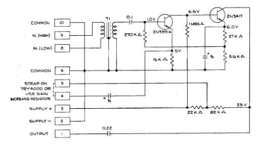
THE AM4100 AMPLIFIER IS PRIMARILY INTENDED FOR USE AS A LOW-IMPEDANCE MICROPHONE PREAMPLIFIER. It is equipped with an input transformer whose primary winding is ungrounded, allowing balanced or unbalanced operation.
