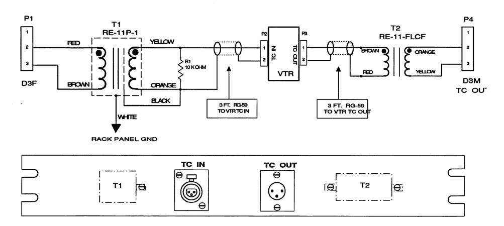
For central time code source in a multi machine environment, quality transformers are needed. Transformers provide, 1) ground loop isolation, 2) keep time code out of the audio and, 3) keep spurious signals out of the time code. If the VTR TC input is 10K or lower, R1 can be omitted. Both transformers are small enough to fit on a 1.75" rack panel mounted directly under the VTR.
