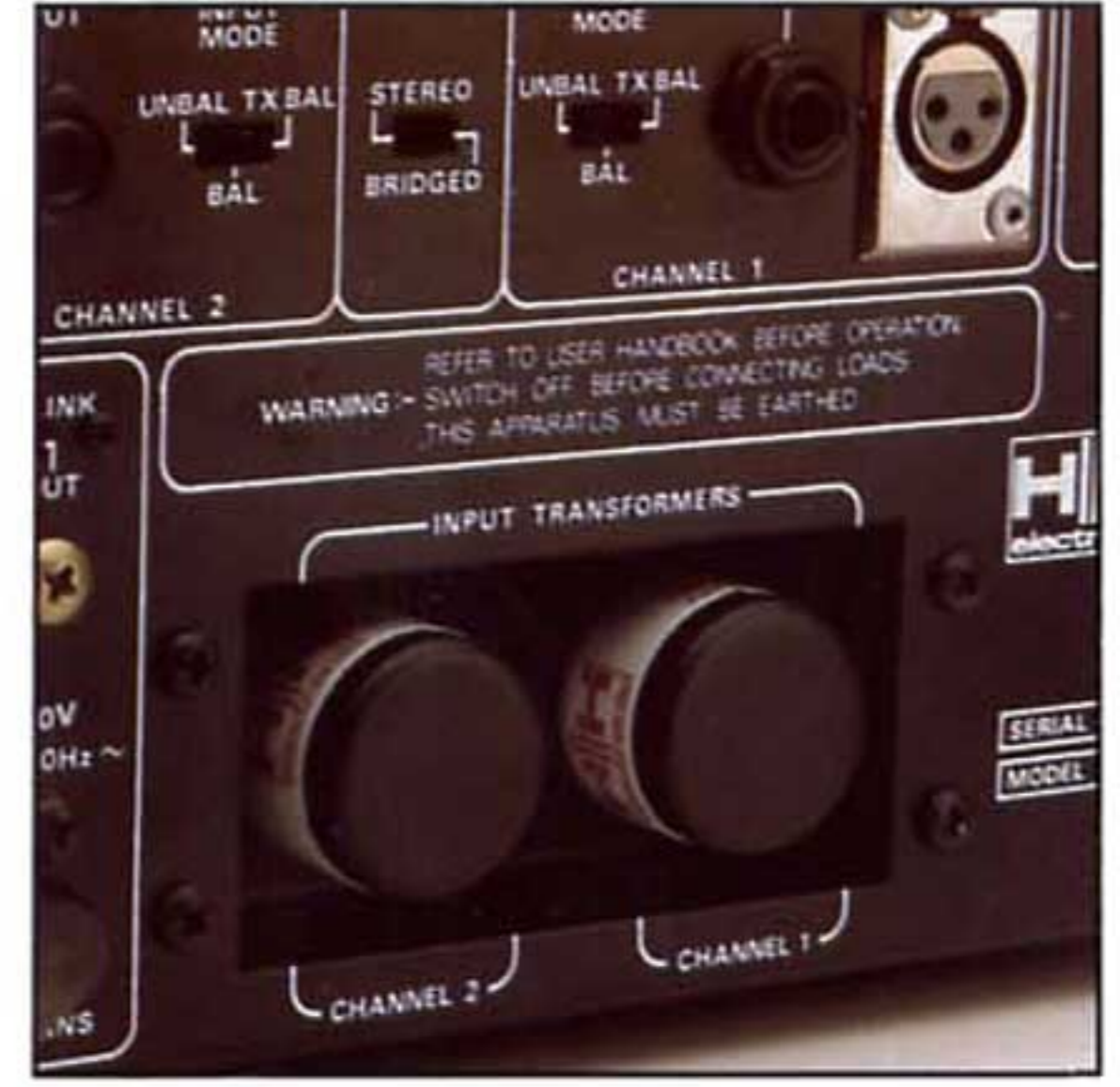
PLUG IN MATCHING TRANSFORMERS AND INPUT MODE SWITCHING FACILITIES
