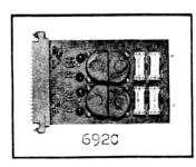
The 692C can be used for changing the gain simultaneously of two channels, using an attenuator per channel, with one remote actuator driving both circuits at once.
