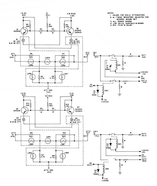
692C DOUBLE ATTENUATOR SCHEMATIC
