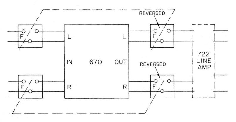
THE FADERS MARKED "F"ARE GANGED 20 STEP- 20 DB BRIDGED "T" FADERS
