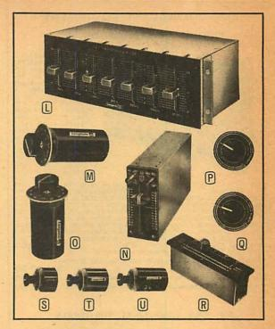
R Langevin Model SPP-2007 Straight Line Pan Pot—For mixing one channel into two. Ladder type with 12 db insertion loss and 180° field. Location of -3 db point at 0°; 90° at extreme right and left. Sixteen steps used per section. For horizontal placement. Supplied with red knob. Size, 6¾" x ½", x ½", x 2¾" d. \$10800 Shpg. Wt., 1 lb. Net Each.
