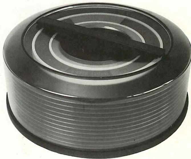
Fig. 3 The disc stack of the CDCBK 6XX contains eleven discs with a diameter of 14" (35.6 cm). Concentric tracks are located on the upper surface of each disc, over which the magnetic heads glide without contact or friction on a cushion of air.
