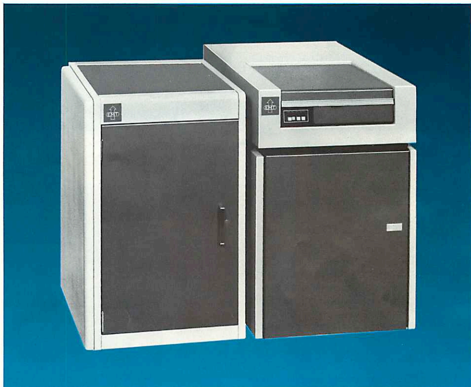
Fig. 1 The prototype of the EMT 450 Digiphon consists of three component units. At the right, the CDC Disc Drive; to the left, the computer. The control unit is shown on page 4.
