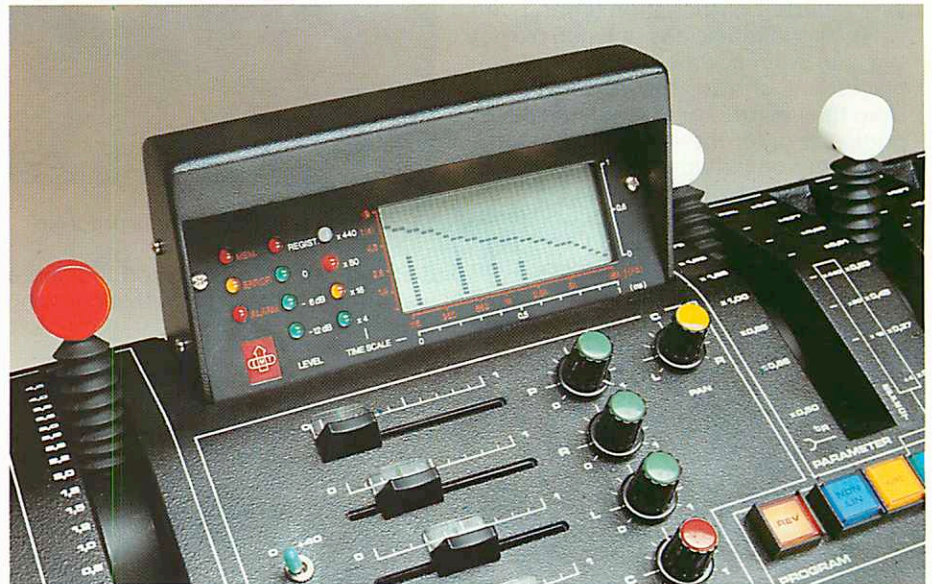
Fig. 3 The selected frequency response of the reverberation time and the amplitude/time distribution of the first reflections are identifiable at a glance on the display of the EMT 251.
