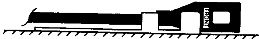
GLM-SM Surface Mount used to make a hypercardioid boundary mic.
