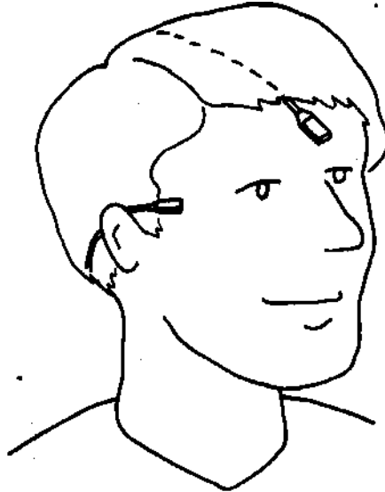
Fig. 3. Two effective GLM placements on a theatrical performer.
