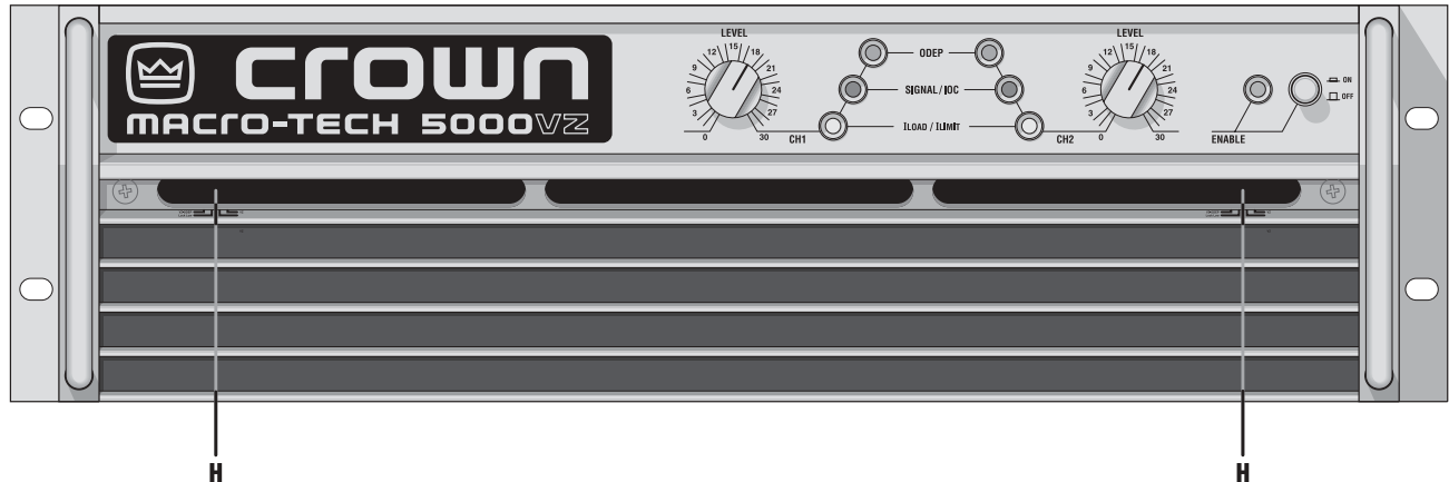
Fig. 2.2 Front Facilities behind the Filter Grille
