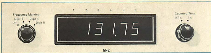
Fig.8. Digital frequency display and the frequency marking and counting time selectors
