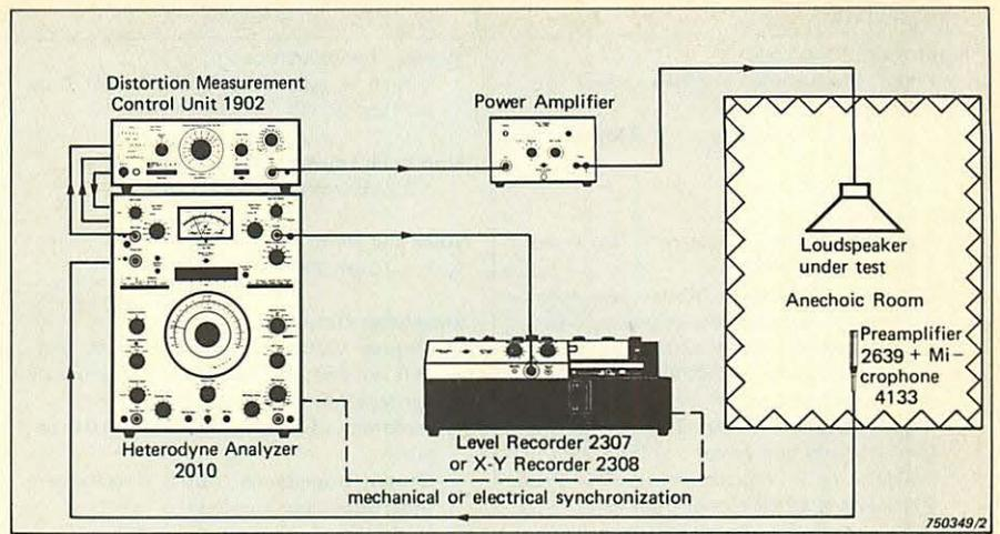
Fig.10. Set-up for recording the distortion characteristics of a loudspeaker
