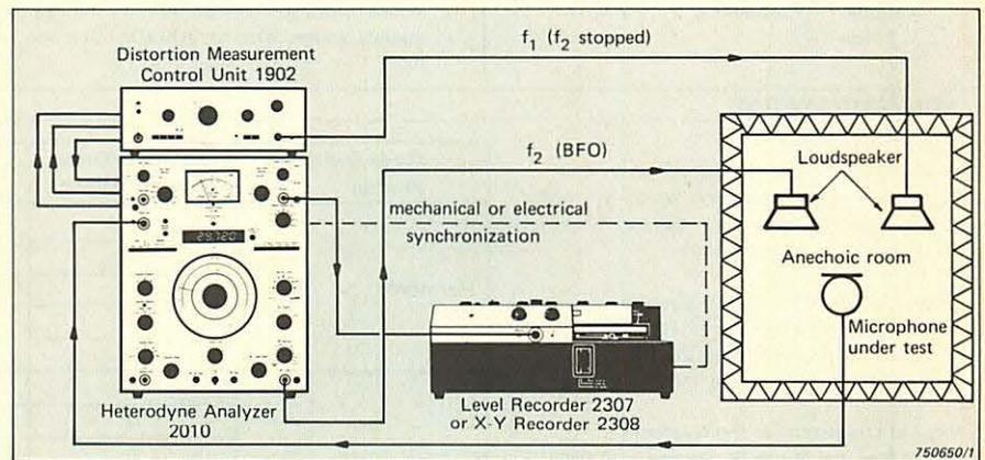
Fig.11. Set-up for recording intermodulation and difference-frequency distortion analyses of a microphone
