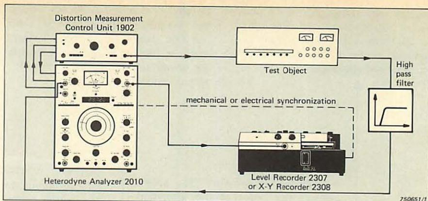
Fig.7. Extending the dynamic range of the 1902/2010 combination in the "Intermodulation" mode by means of a simple, high pass filter
