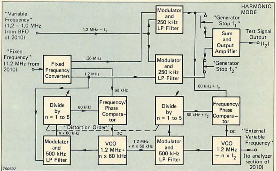
Fig.2. Simplified block diagram of the 1902 in the "Harmonic" mode
