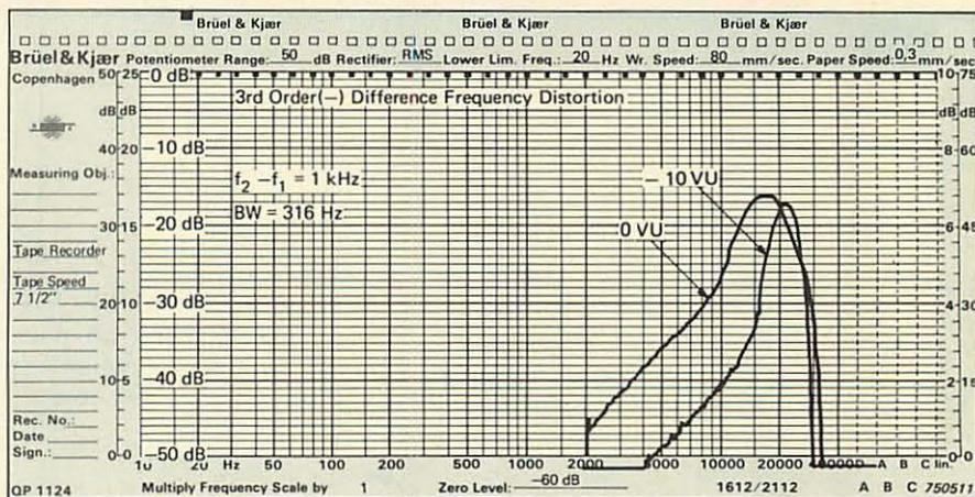
Fig.9. Difference-frequency analysis recorded with the set-up in Fig.8
