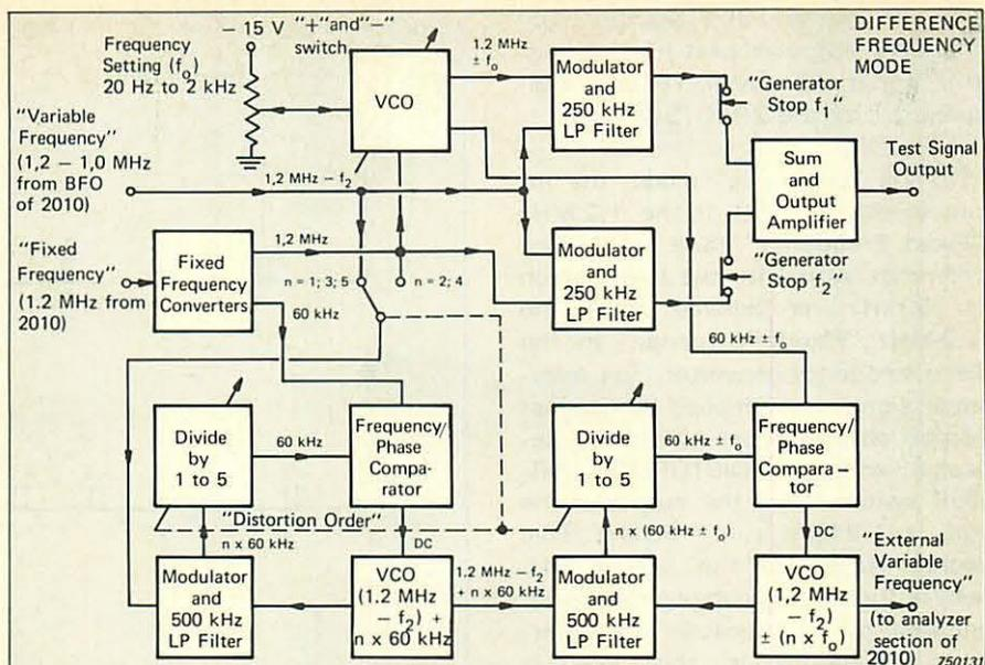
Fig.3. Simplified block diagram of the 1902 in the "Difference-frequency" mode
