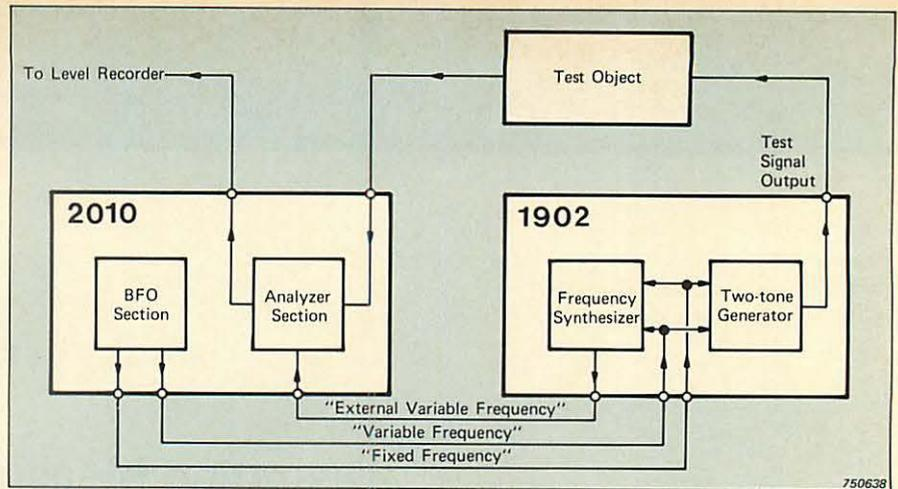
Fig.1. Interconnection of Type 1902 and Type 2010
