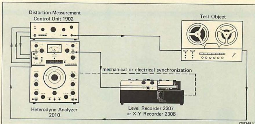
Fig.8. Set-up for analysis of distortion on a tape recorder
