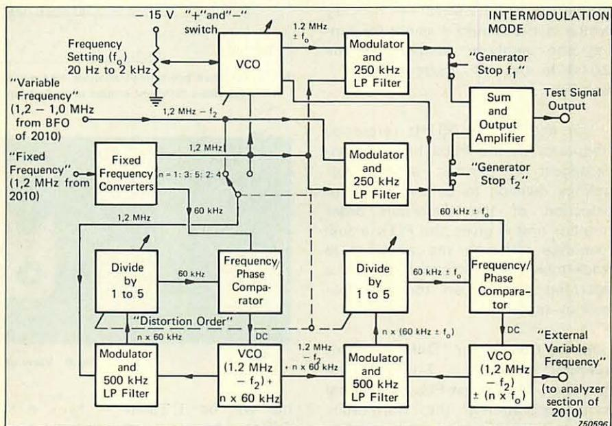
Fig.4. Simplified block diagram of the 1902 in the "Intermodulation" mode
