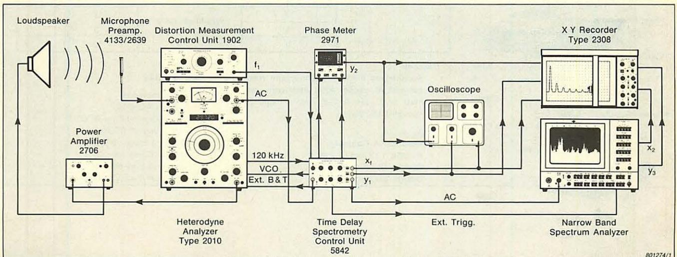
Fig. 12. Setup including the Time Delay Spectrometry Control Unit Type 5842 for free field loudspeaker measurements in ordinary environments
