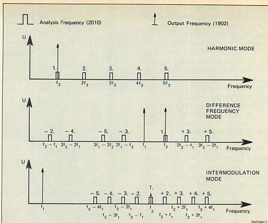
Fig.5. Relative position of analysis frequencies of 2010, and test signal frequencies of 1902 in the three different modes of operation
