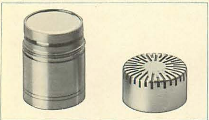
Fig. 3. 1/2" Microphone Type 4155 with protection grid removed. The diaphragm is flat and practically flush with the housing. This allows frequency response calibration to be performed using the Electrostatic Actuator UA 0033
