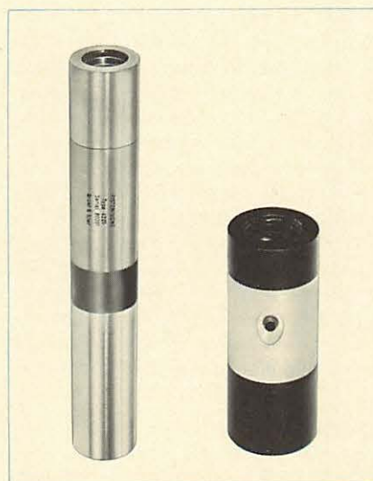
Fig. 17. Pistonphone Type 4220 and Sound Level Calibrator Type 4230
