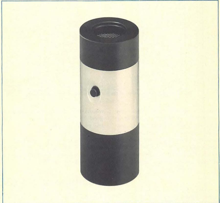
The Sound Level Calibrator Type 4230 is a pocket sized, battery operated sound source intended for quick and direct calibration of sound level meters and other sound measuring systems. It is designed to fit B & K 1" and 1/2" microphones, but with the correct adaptors it can be used for 1/4" and 1/8" microphones as well.
