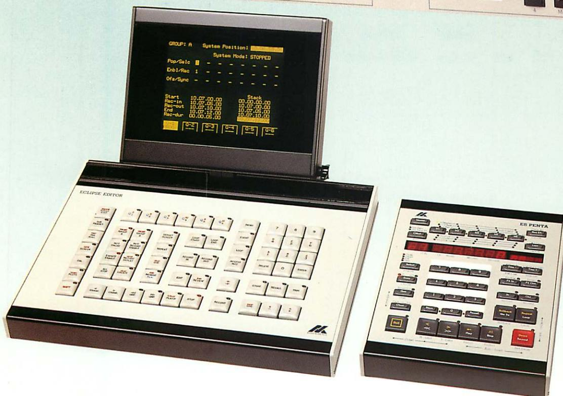
Audio Kinetics ES.Lock fundamentally offers the ability to interface, control and synchronise any one tape recorder to a number of other machines. But the real power of ES.Lock is to extend control and synchronisation to complex networks of audio, video and film machines and peripheral studio systems - with swift, silent efficiency and complete dependability.
