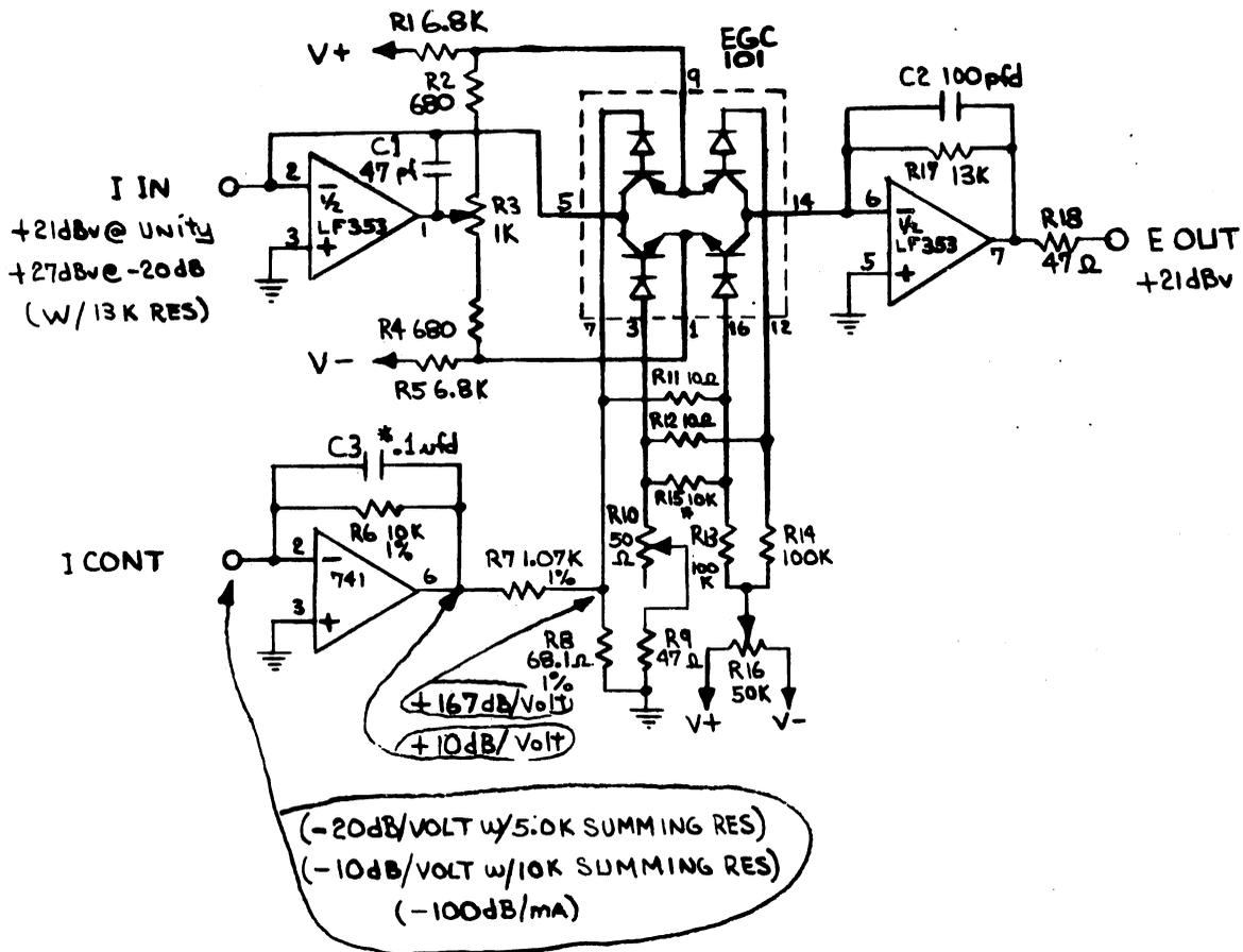
EGC-205M (FULLY TRIMMED VCA CKT WITH CURRENT INPUTS & VOLTAGE OUTPUT)
