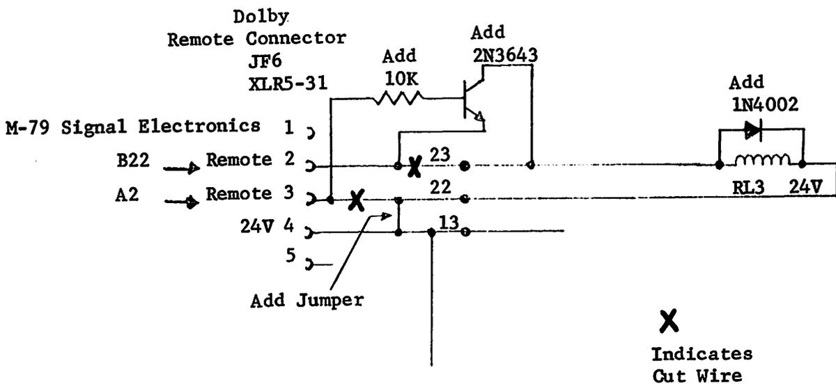
NOTE: Added Circuit may be mounted on a Vector Board inside the DOLBY unit.
