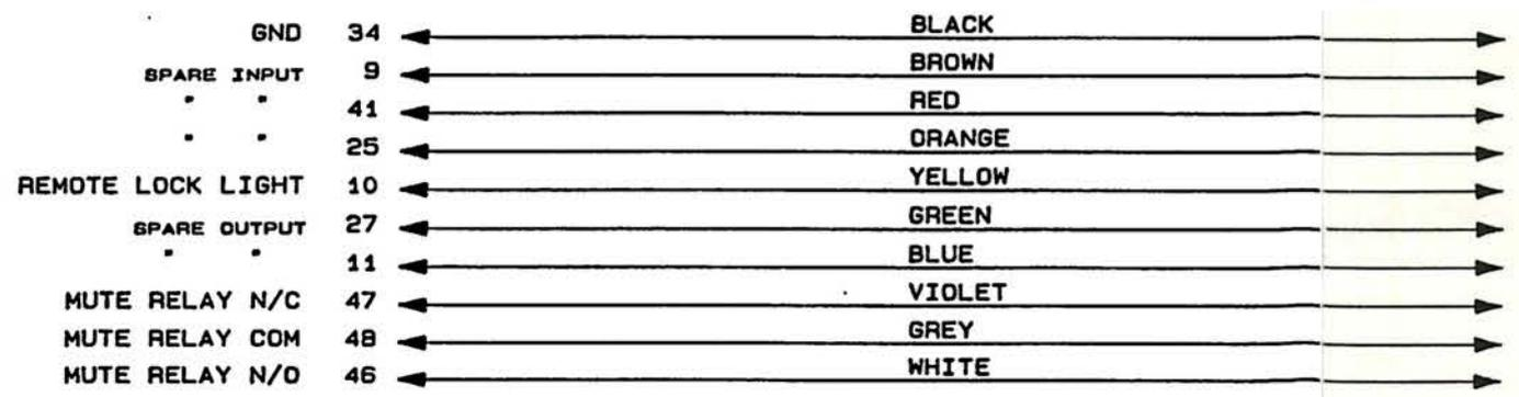
UNCONNECTED 6" PIGTAIL FOR CUSTOMER CONNECTION
