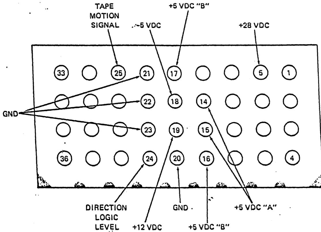
Figure 3. Remote Cable Connector (Control Unit Disconnected)
